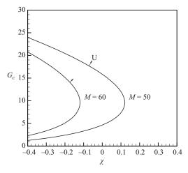
FIGURE 3. Critical Galileo number  $G_c$  as a function of the Soret number  $\chi$  for the streamwise instabilities in the long-wave limit (3.3) for different Marangoni numbers. The arrows indicate the unstable side of the curves. It is shown that above a certain value of  $\chi$  the situation is long-wave unstable for any Galileo number (Ka = 500, Pr = 10, L = 0.01, B = 0.02,  $\beta = 15^{\circ}$ ); relation (3.3) is independent of Ka, Pr, and L.
