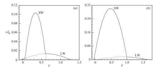
FIGURE 18. Growth rate  $\omega_{0i}^{v}$  as a function of the ray velocity V for both long-wave (LW) and short-wave (SW) streamwise instabilities and for  $\chi = 0$  and M = 245: (a) G = 2.8; (b) G = 4. The branches of saddle points which determine the properties of the spatio-temporal instability are indicated by solid lines (Ka = 500, Pr = 10, L = 0.01, B = 0.02,  $\beta = 15^{\circ}$ ).
