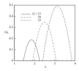
FIGURE 13. Growth rate  $\omega_{0i}^{v}$  as a function of the ray velocity V for the streamwise short-wave thermocapillary instability (P-mode) and for different Galileo numbers G,  $\chi = 0$ , and M = 100 (Ka = 500, Pr = 10, L = 0.01, B = 0.02,  $\beta = 15^{\circ}$ ).
