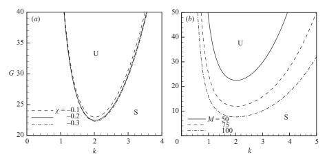
FIGURE 8. Neutral curves for the oscillatory spanwise short-wave instabilities in the G-k parameter space: (a) neutral curves for different Soret numbers  $\chi$  and M = 50; (b) neutral curves for different Marangoni numbers M and  $\chi = -0.2$  (Ka = 500, Pr = 10, L = 0.01, B = 0.02,  $\beta = 15^{\circ}$ ).
