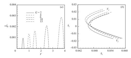
FIGURE 9. (a) Growth rate  $\omega_{0i}^v$  as a function of the ray velocity V and (b) loci of the unstable contributing saddle points in the k-plane, for the streamwise long-wave instability (merged S-and H-modes) and for different Galileo numbers G,  $\chi = 0$ , and M = 100. In (b),  $V_r$  and  $V_l$  refer to the right and left boundaries of the unstable ray domains (Ka = 500, Pr = 10, L = 0.01, B = 0.02,  $\beta = 15^\circ$ ).
