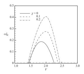
FIGURE 15. Growth rate  $\omega_{0i}^{v}$  as a function of the ray velocity V for the streamwise short-wave thermocapillary instability (P-mode) and for different Soret numbers  $\chi$ , M = 100, and G = 15 (Ka = 500, Pr = 10, L = 0.01, B = 0.02,  $\beta = 15^{\circ}$ ).
