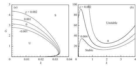
FIGURE 5. Neutral curves for the stationary spanwise instabilities in the G-k parameter space for different Soret numbers  $\chi$  and M = 50: (a) neutral curves for the long-wave S-mode; (b) neutral curves for the P-mode, which merge with the curves of the S-mode for  $\chi = 0.004$ (Ka = 500, Pr = 10, L = 0.01, B = 0.02,  $\beta = 15^{\circ}$ ).
