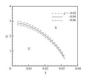
FIGURE 7. Neutral curves for the oscillatory spanwise long-wave instabilities in the G-k parameter space for different Soret numbers  $\chi$  and M = 50 (Ka = 500, Pr = 10, L = 0.01, B = 0.02,  $\beta = 15^{\circ}$ ).
