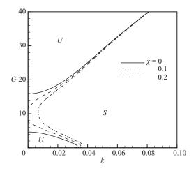
FIGURE 2. Neutral curves for the streamwise instabilities in the G-k parameter space for different Soret numbers  $\chi$  and M = 50. The upper unstable domain of the H-mode instability and the lower unstable domain of the S-mode instability merge when  $\chi$  is increased (Ka = 500, Pr = 10, L = 0.01, B = 0.02,  $\beta = 15^{\circ}$ ). U denotes an unstable domain and S a stable one.
