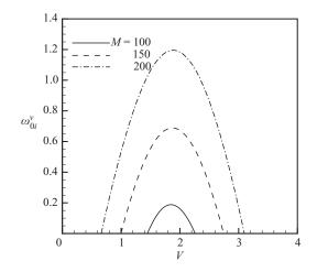
FIGURE 14. Growth rate  $\omega_{0i}^{v}$  as a function of the ray velocity V for the streamwise short-wave thermocapillary instability (P-mode) and for different Marangoni numbers M,  $\chi = 0$ , and G = 15 (Ka = 500, Pr = 10, L = 0.01, B = 0.02,  $\beta = 15^{\circ}$ ).
