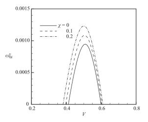
FIGURE 11. Growth rate  $\omega_{0i}^{v}$  as a function of the ray velocity V for the streamwise long-wave instability (merged S- and H-modes) and for different Soret numbers  $\chi$ , M = 100, and G = 2 (Ka = 500, Pr = 10, L = 0.01, B = 0.02,  $\beta = 15^{\circ}$ ).
