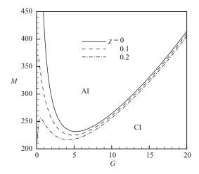
FIGURE 16. AI/CI boundary curves in the M-G parameter space for the streamwise short-wave thermocapillary instability (P-mode) and for different Soret numbers  $\chi$  (Ka = 500, Pr = 10, L = 0.01, B = 0.02,  $\beta = 15^{\circ}$ ).
